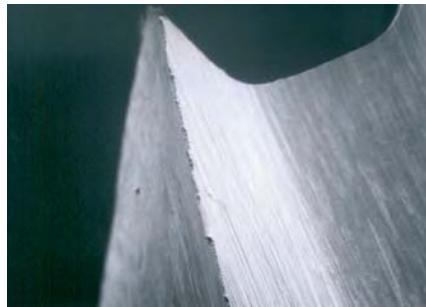
Surface of a conventional fluteless tap
